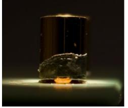
**Figure 1:** PCB Connector with PTFE tilting and lifting off board during reflow.
